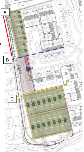
One way is to lay a land drain and backfill with stone to leave a solid surface (B to C). Or we erect a suitable sturdy fence or barrier along the side where the ditch is. Both will be costly, but if the stone option is used, we will gain space. It is recommended to pipe and stone the ditch, it will only need doing once whereas a fence or barrier would need to be maintained and replaced over time.
